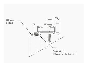
Having manufactured and installed the window so that there is a 5mm gap (approx.) between mainframe and masonry, it may be necessary to insert a flexible foam strip to form a base for the silicone sealant.
