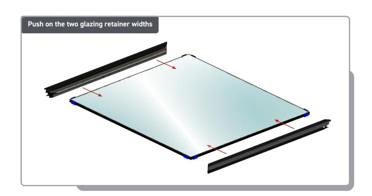
Ensure the corner key is correct way up and cleat aligns. Then fit the two glazing retainer lengths
