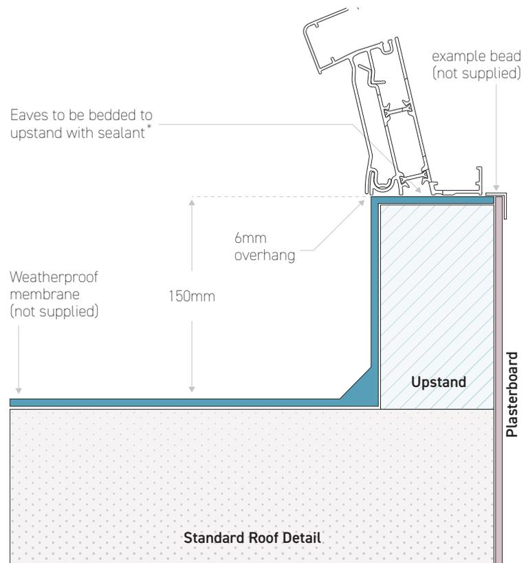
\* Sealant to be applied to the underside of the eaves as per installation guide instructions only
