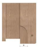
Extra cut-out section on Bottom Sash for friction hinge
