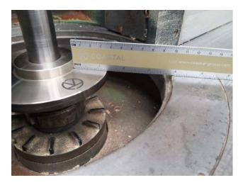
Setting Gauge is placed on the bottom of the spindle shaft with the logo in the up position to determine the bed height as shown above.
