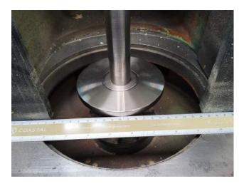
Setting Gauge is then removed and turned over and this becomes the setting point for the fences.
