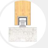
Note: Bottom Roller Guide can also be mounted on floor and channel rebated into bottom of door leaf. Ideal for use as Room Dividers
