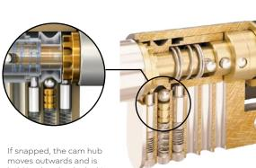
If snapped, the cam hub moves outwards and is held in place by the locking pins. Lock can still be opened inside using the key or thumbturn.
