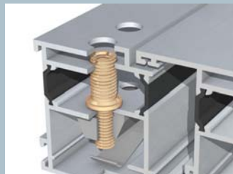
Screw support stud screw with mounting plate (special screwdriver). Recommended tightening torque 12 to max. 17 Nm. The collar should rest on the main chamber.
