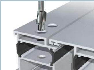
Use Hahn counterbore to drill out the 11 mm-diameter holes to a 15 mm diameter. Do not drill through main chamber.
